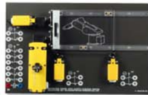
Protective door monitoring switch
